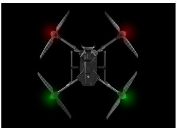
The red light indicates the front of the E900 drone, while the green light indicates the rear.
