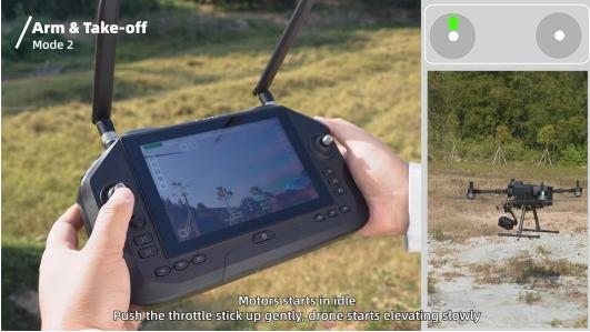
6. When descent is needed, slowly pull the throttle stick down to allow the aircraft to descend gently to a flat surface.
