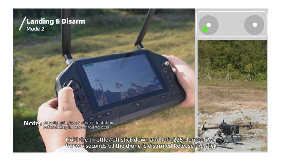
8. After the aircraft has stopped, turn off the aircraft and remote controller power in sequence.
