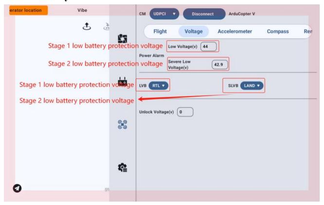
To prevent unnecessary risks caused by insufficient battery power, the aircraft will identify whether low battery protection behavior should be triggered based on the set protection voltage. If the user does not make a selection within 10 seconds, the aircraft will automatically enter return-to-home (RTH) mode after 10 seconds. During the return process, the user can briefly press the return-to-home button on the remote controller or switch to another flight mode to cancel the return.
