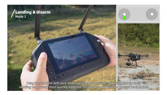
7. After landing, pull the throttle stick to the lowest position and wait for the drone to enter idle mode. Lock it in place until the motors stop.
