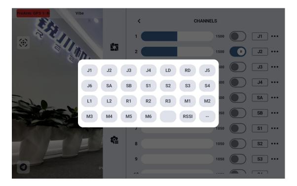
Select the target channel, click the channel mapping button, the pop-up switch list, select the required switch, you can successfully connect.
