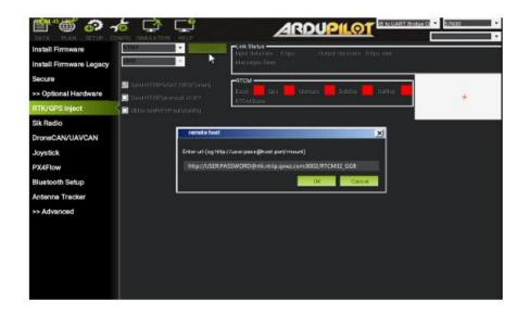
Among them, USER is the FindCM service account name applied by the user, PASSWORD is the corresponding password, rtk.ntrip.qxwz.com is the FindCM service address of qianhe location server, 8002 port broadcasts WGS84 coordinate system data, and RTCM32\_GGB is the data source for externally broadcasting RTCM3.2 format data.
